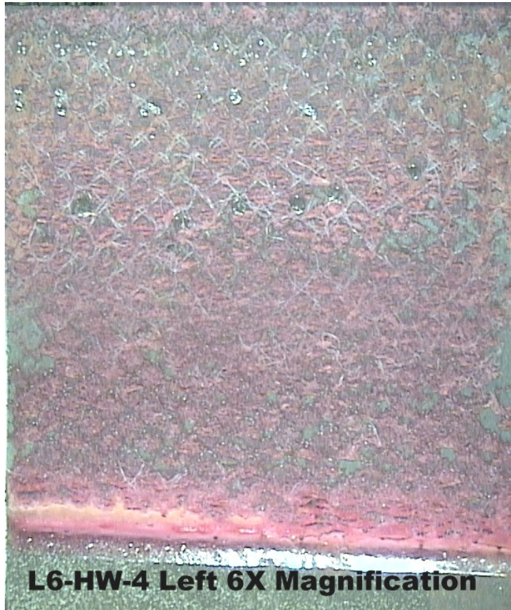
Cohesive Fracture of Adhesive Film (Option 6 silane treatment)
